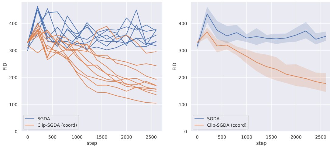
Figure 17: FID curves when training StyleGAN2 for 2600 kings (thousands of images seen by the discriminator) with SGDA and clipped-SGDA (coordinate), corresponding to the hyperparameters in Tables 8 & 9 respectively. The left figure is the individual runs for each choice of hyperparameters, and the right is the mean and 95% confidence interval of these runs. Every SGDA-trained model for the wide range of learning rates we tried failed to improve the FID, while models trained with clipped-SGDA (with appropriately set hyperparameters) are generally able to learn some meaningful features and improve the FID.
